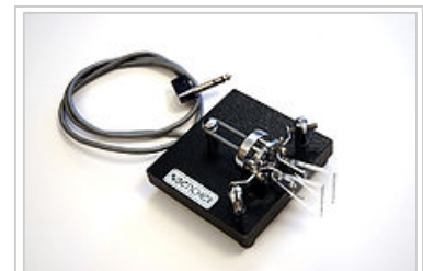
A commercially manufactured iambic paddle used in conjunction with an electronic keyer to generate high-speed Morse code, the timing of which is controlled by the electronic keyer. Manipulation of dual-lever paddles is similar to the Vibroplex, but pressing the right paddle generates a series of dahs , and squeezing the paddles produces dit-dah-dit-dah sequence. The actions are reversed for left-handed operators.
