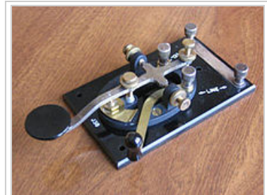
Typical "straight key". This U.S. model J-38, was manufactured in huge quantities during World War II. The signal is "on" when the knob is pressed, and "off" when it is released. Length and timing of the dots and dashes are entirely controlled by the telegraphist.
