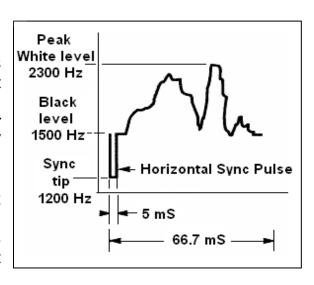
• SSTV is **not** a digital mode like RTTY and PSK31. It is an analogue mode like SSB. It uses frequency modulation, whereby every different value of brightness
